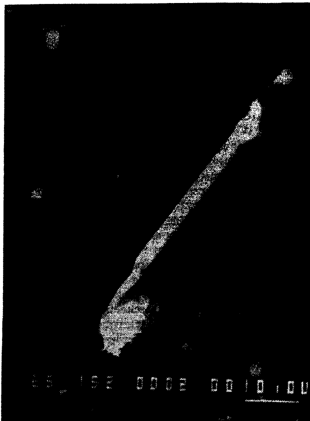
Figure 2. Linearly shaped particle rich in Na and Cl at the end a Si-rich particle.
